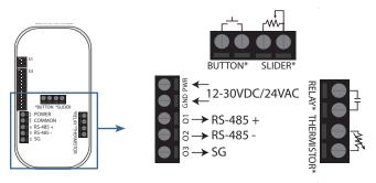
NOTE: A 120  $\Omega$  termination resistance may be added in parallel with the RS-485 +/- by moving the very top DIP switch (DIP 1) to the left position. See "DIP Configuration" section for more information.
